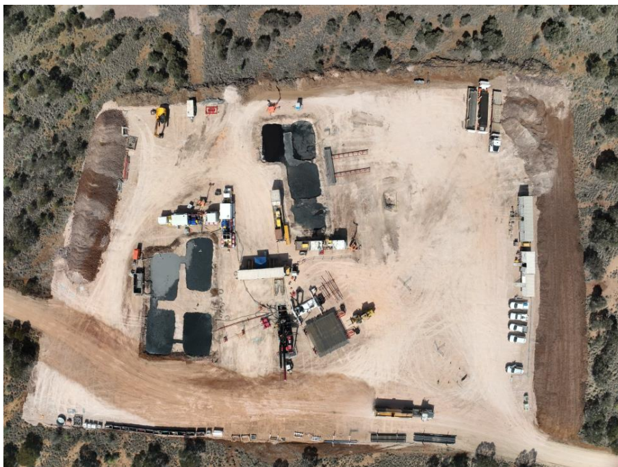
Image 2.2 Example of drill pad arrangement
