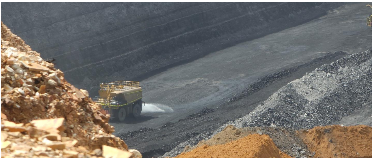
Plate 22 Water cart in operation at Pit 6
