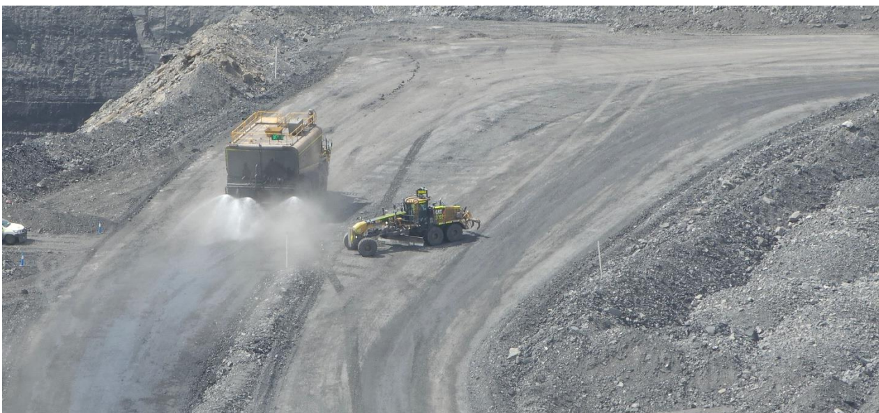
Plate 23 Water cart in operation on haul road at Pit 6
