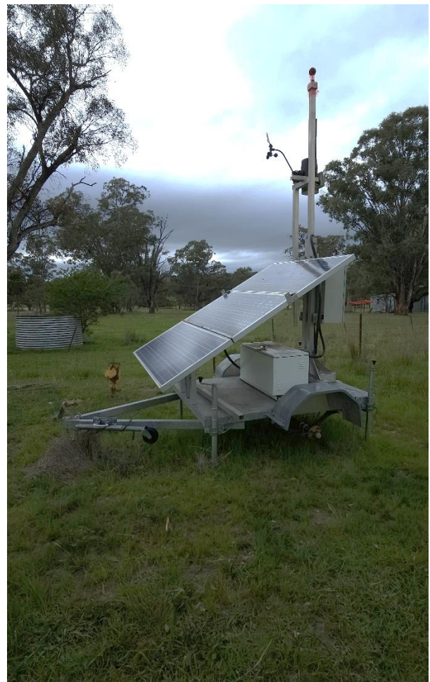
Plate-14 Fixed real-time noise monitor in village of Wollar
