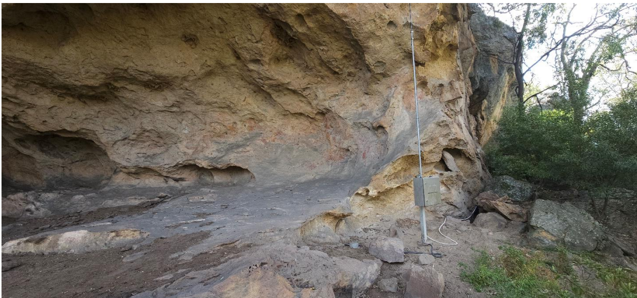
Plate 10 Fixed blast monitor at Castle Rock (Site 72)
