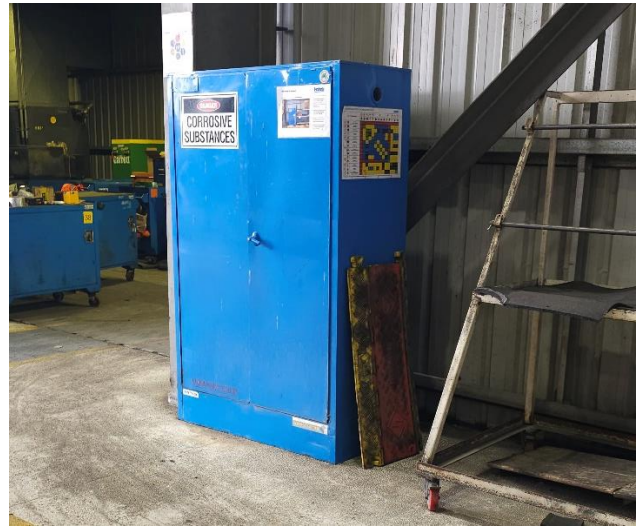
Plate 7 Locked corrosive substances storage available at workshop
