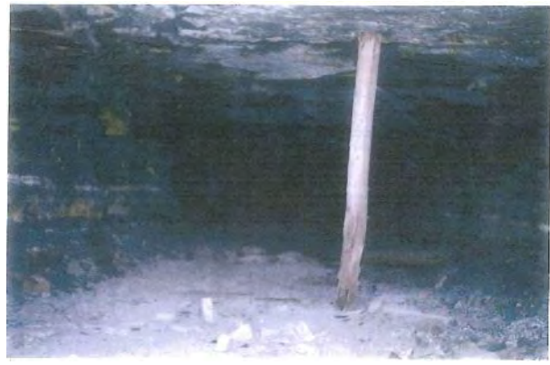
Plate 6: single wooden roof support of mined shale deposit (source: Niche 2015).
