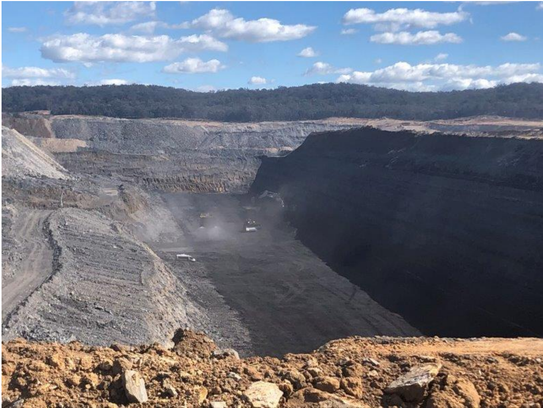
Plate 25 – Pit 6 water cart entering pit bottom to suppress evident dust production
