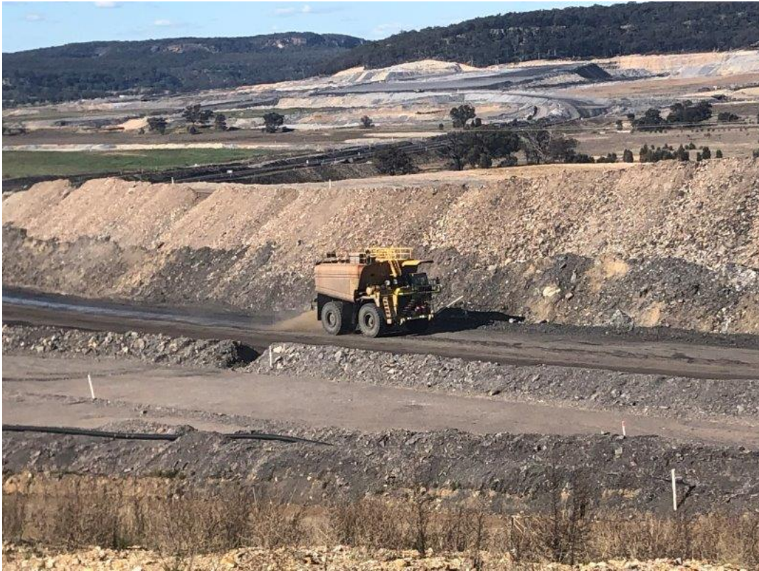
Plate 29 – Water cart active on haul roads utilising dust suppressant compound
