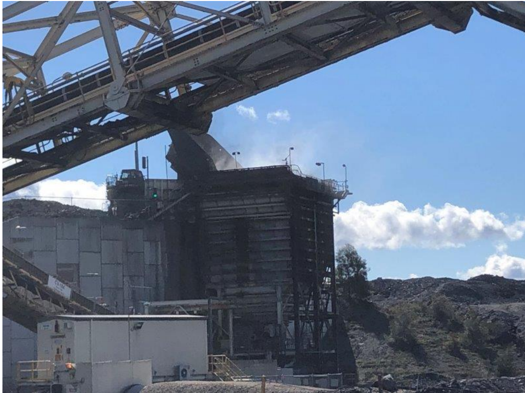
Plate 9 – Sprays operational to raw coal dump
