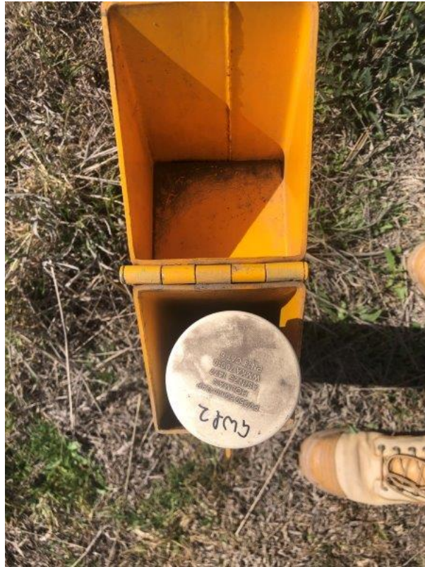
Plate 23 – Groundwater monitoring well GW02
