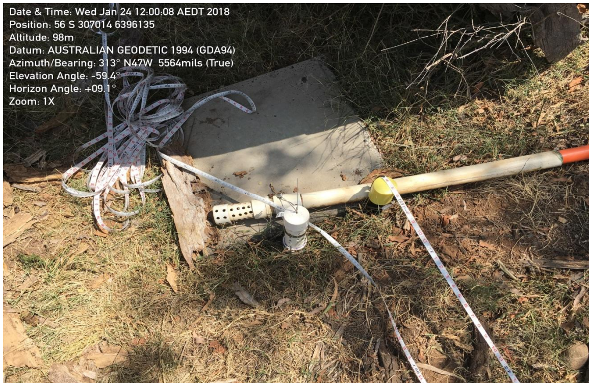
Figure 3 Re-Located Flow Monitoring Station 1 North Wambo Creek Sensor and Backup Sensor in relation to the Stream Bed – January 2018.
