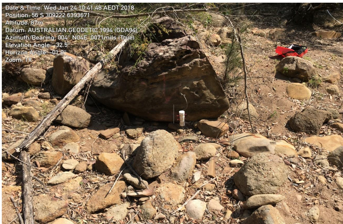
Figure 6 New Flow Monitoring Station (Upper North Wambo Creek) Sensor in relation to the Stream Bed – January 2018.
