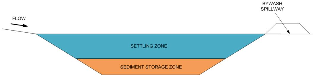
Below is an indicative overview of the required footprint area needed to construct a sediment basin, however advice from a competent person shall be sought to accurately determine the sizing prior to construction commencing.
