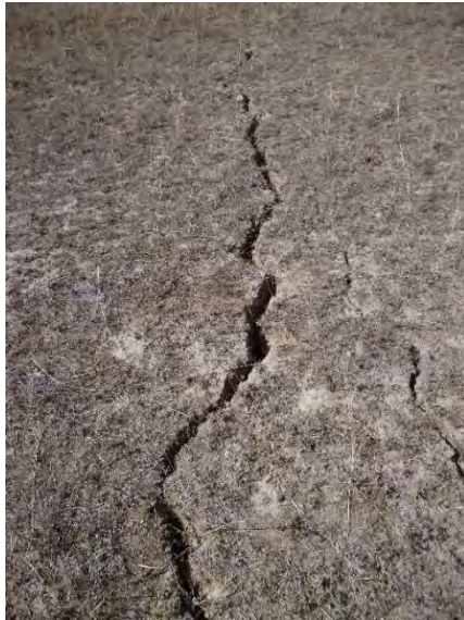
Figure 3-5. Cracking at Surface Over LW 17 (MSEC, 2022)
