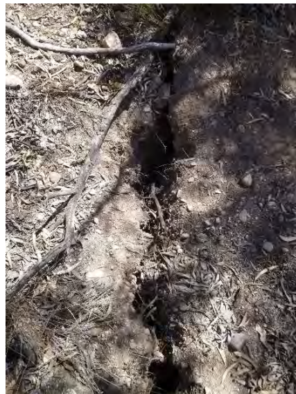
Figure 3-6. Large Crack Development Example Over LW 17 (MSEC, 2022)
