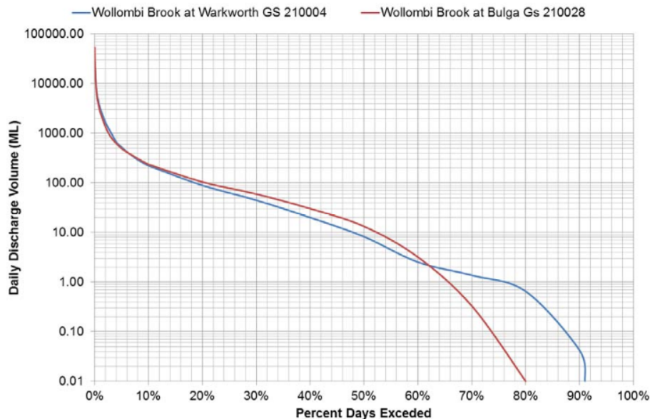
Figure 6: Flow Duration Curves Wollombi Brook Upstream and Downstream of the Mine
