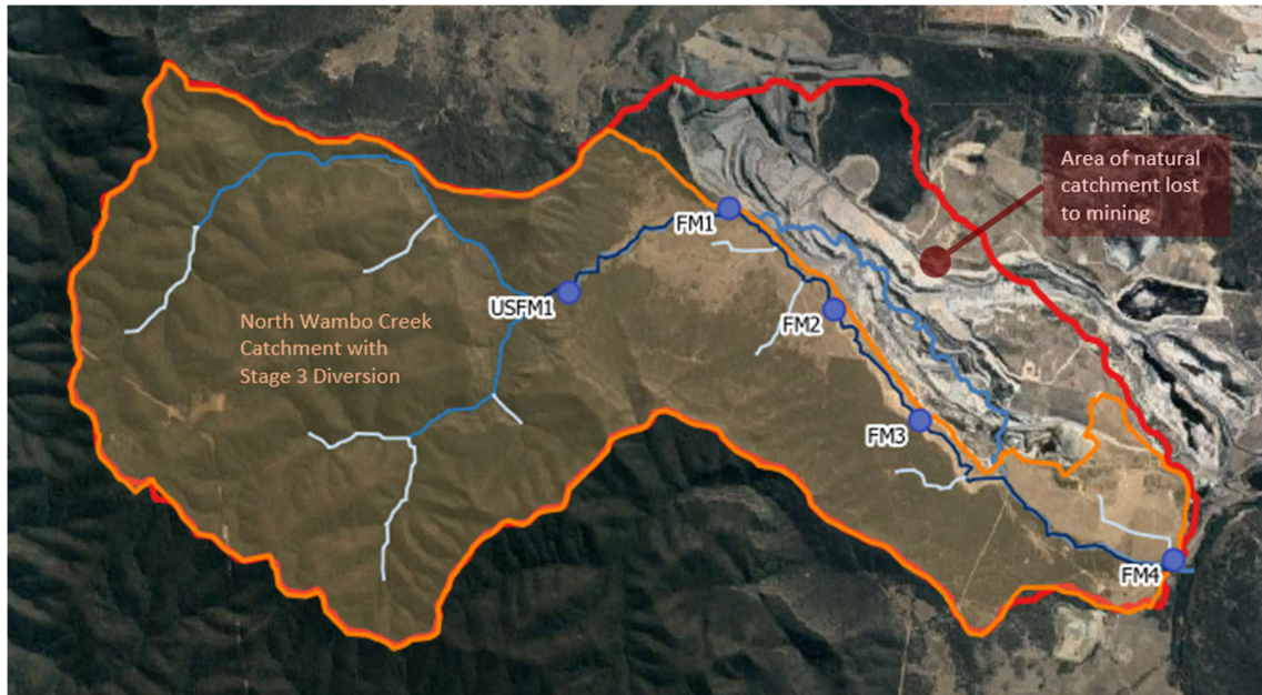
Figure 4: North Wambo Creek Surface Flow Monitoring Locations and Reduction in Catchment Area post Stage 3 Diversion.
