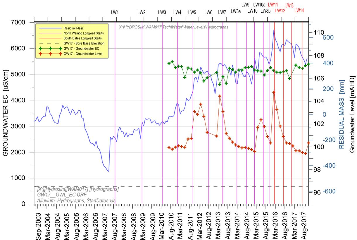
Figure 6. North Wambo Creek Observed and Smoothed Hydrographs and EC at Monitoring Bores GW17
