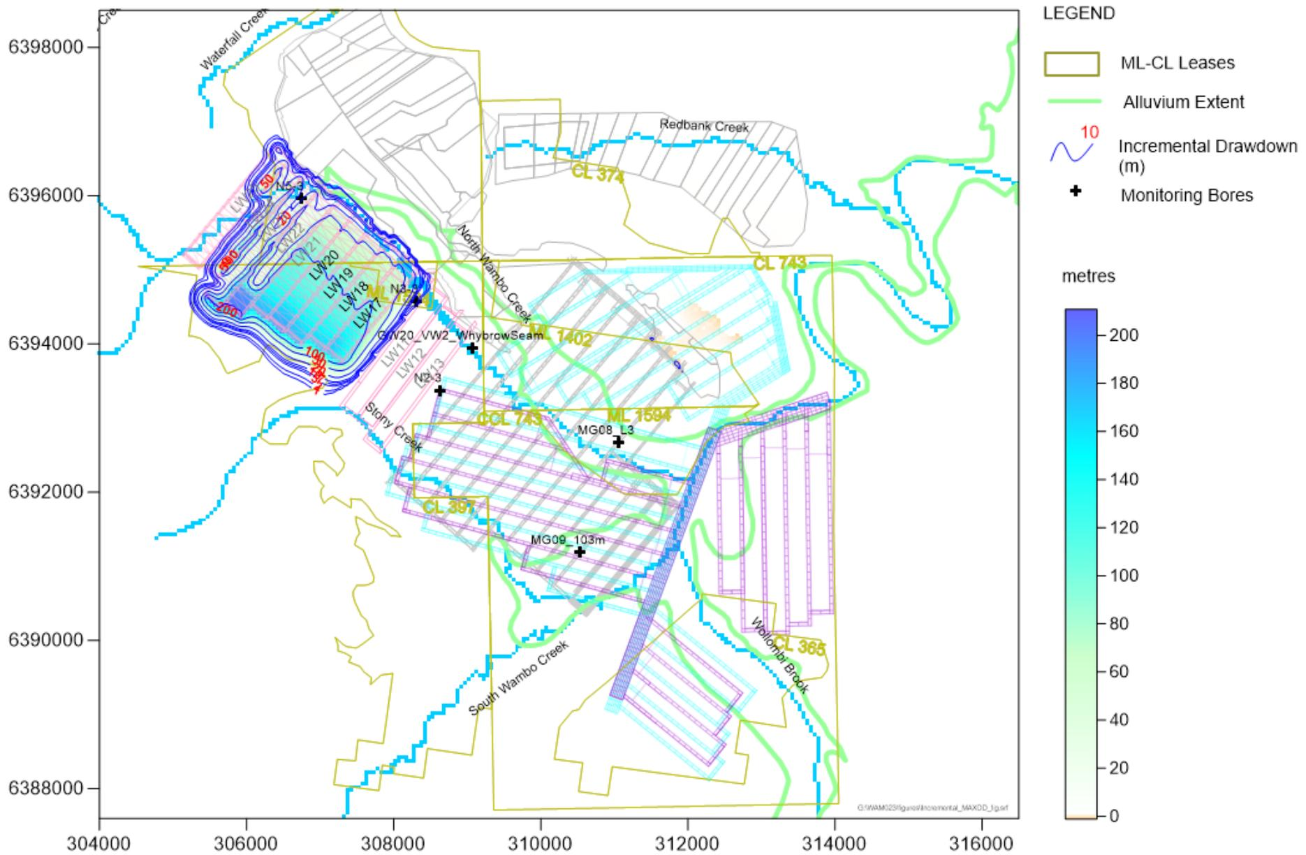
Figure 12. Incremental Maximum Drawdown (m) in Whybrow Seam during Longwalls 17 to part of 22 Mining (SP32-SP36)
