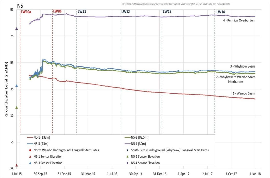
Figure 10. Observed Hydrographs at VWP Monitoring Bore N5
