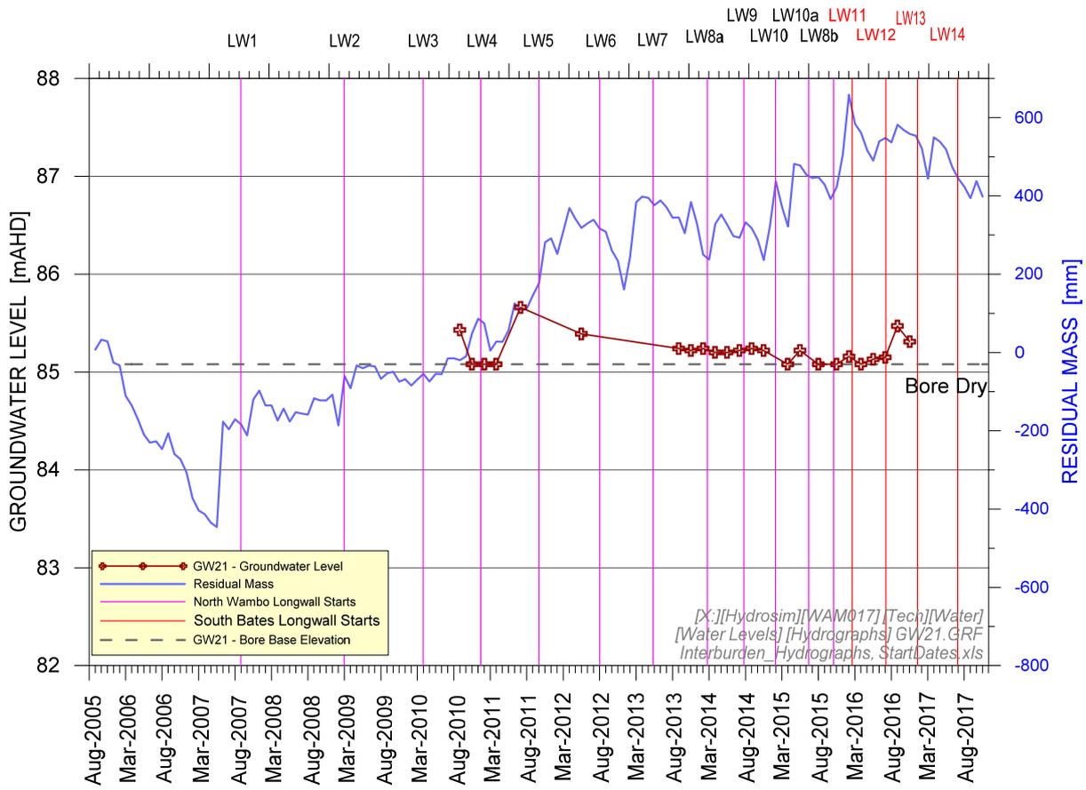
Figure 7. Interburden Observed Hydrograph at Monitoring Bore GW21
