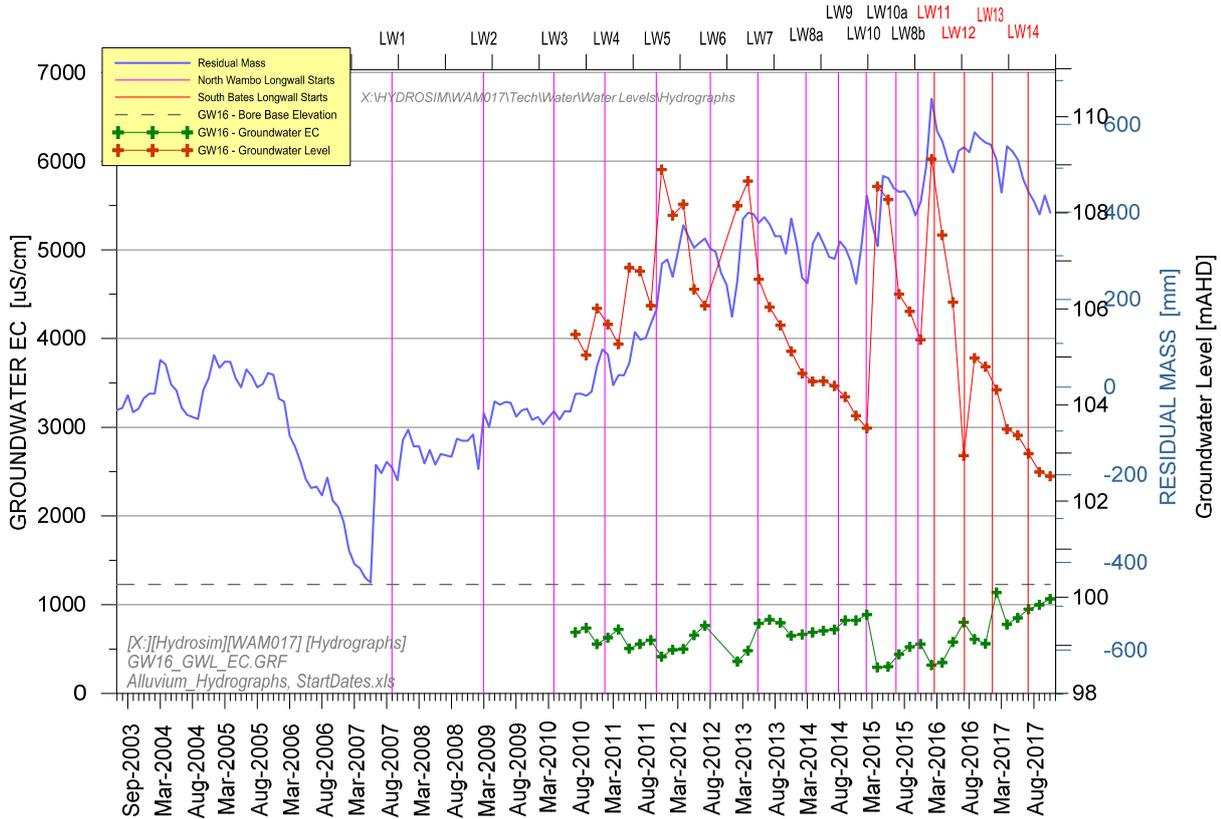
Figure 5. North Wambo Creek Observed and Smoothed Hydrographs and EC at Monitoring Bores GW16
