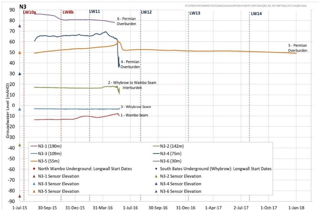
Figure 9. Observed Hydrographs at VWP Monitoring Bore N3
