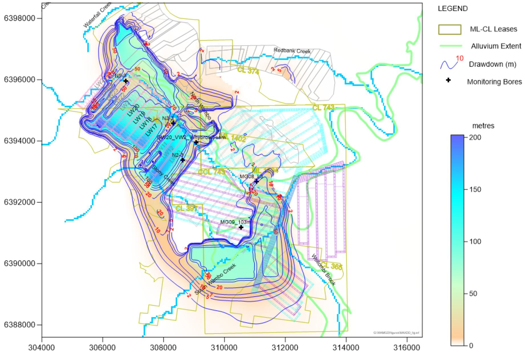
Figure 11. Cumulative Maximum Drawdown (m) in Whybrow Seam during Longwalls 17 to part of 22 Mining (SP32-SP36)
