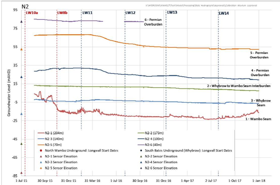
Figure 8. Observed Hydrographs at VWP Monitoring Bore N2
