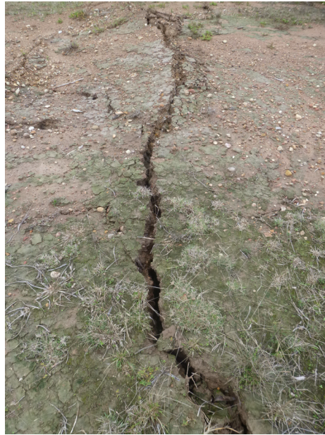
Fig. 4.5 Surface cracking along the North Wambo Creek Diversion due to WYLW11
