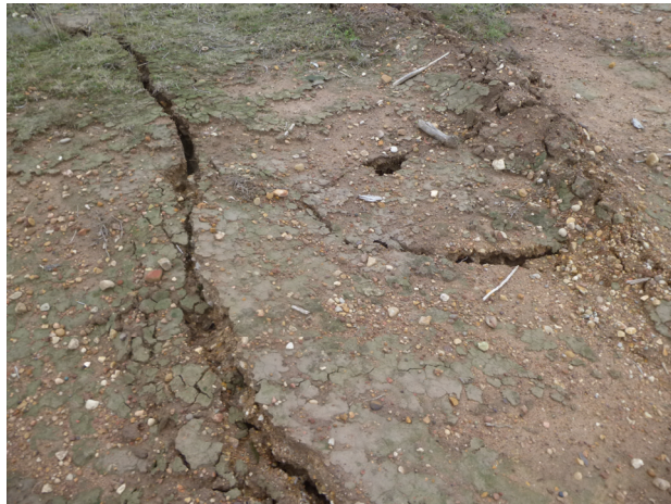
Fig. 4.6 Compression heaving along the North Wambo Creek Diversion due to WYLW11
