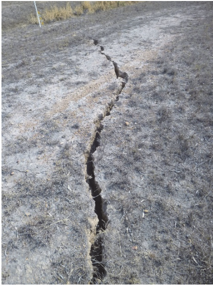
Fig. 4.7 Surface cracking above the middle of WYLW17
