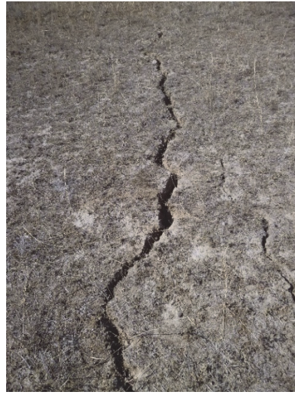
Fig. 4.4 Surface cracking above north-eastern end of WYLW17
