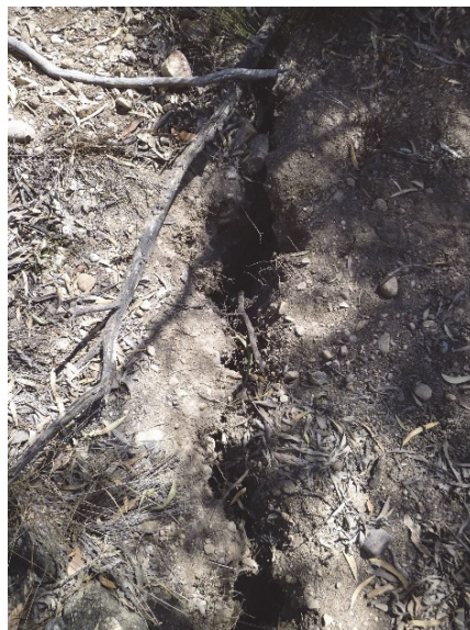
Fig. 4.8 Surface cracking on the steep slopes above the south-western end of WYLW17
