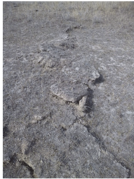
Fig. 4.5 Compression heaving above north-eastern end of WYLW17
