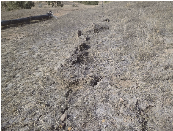
Fig. 4.5 Compression heaving above north-eastern end of WYLW17
