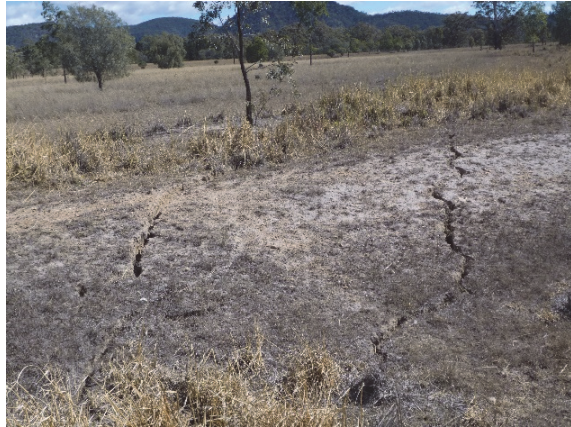
Fig. 4.7 Surface cracking above the middle of WYLW17
