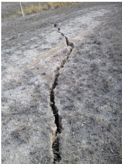
Fig. 4.16 Surface cracking above the middle of WYLW17
