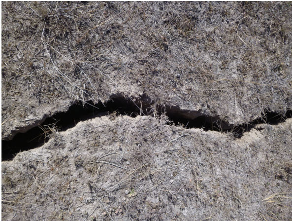
Fig. 4.13 Surface cracking above north-eastern end of WYLW17
