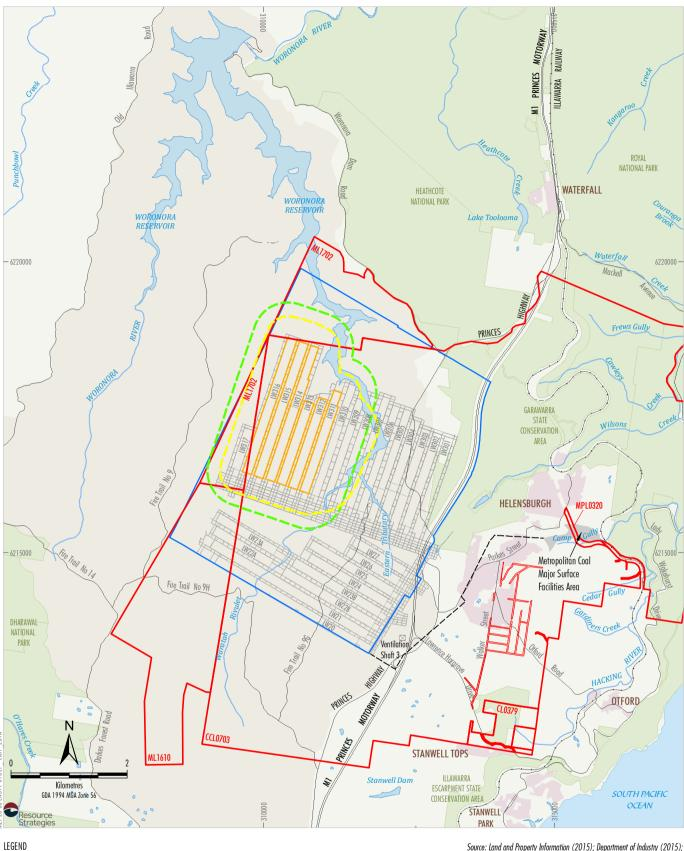
Mining Lease Boundary Woronora Special Area Railway Project Underground Mining Area Longwalls 20-27 and 301-317 Longwalls 311-316 Secondary Extraction Longwalls 311-316 35° Angle of Draw and/or Predicted 20 mm Subsidence Contour 600 m from Longwalls 311-316 Secondary Extraction Existing Underground Access Drive (Main Drift)
