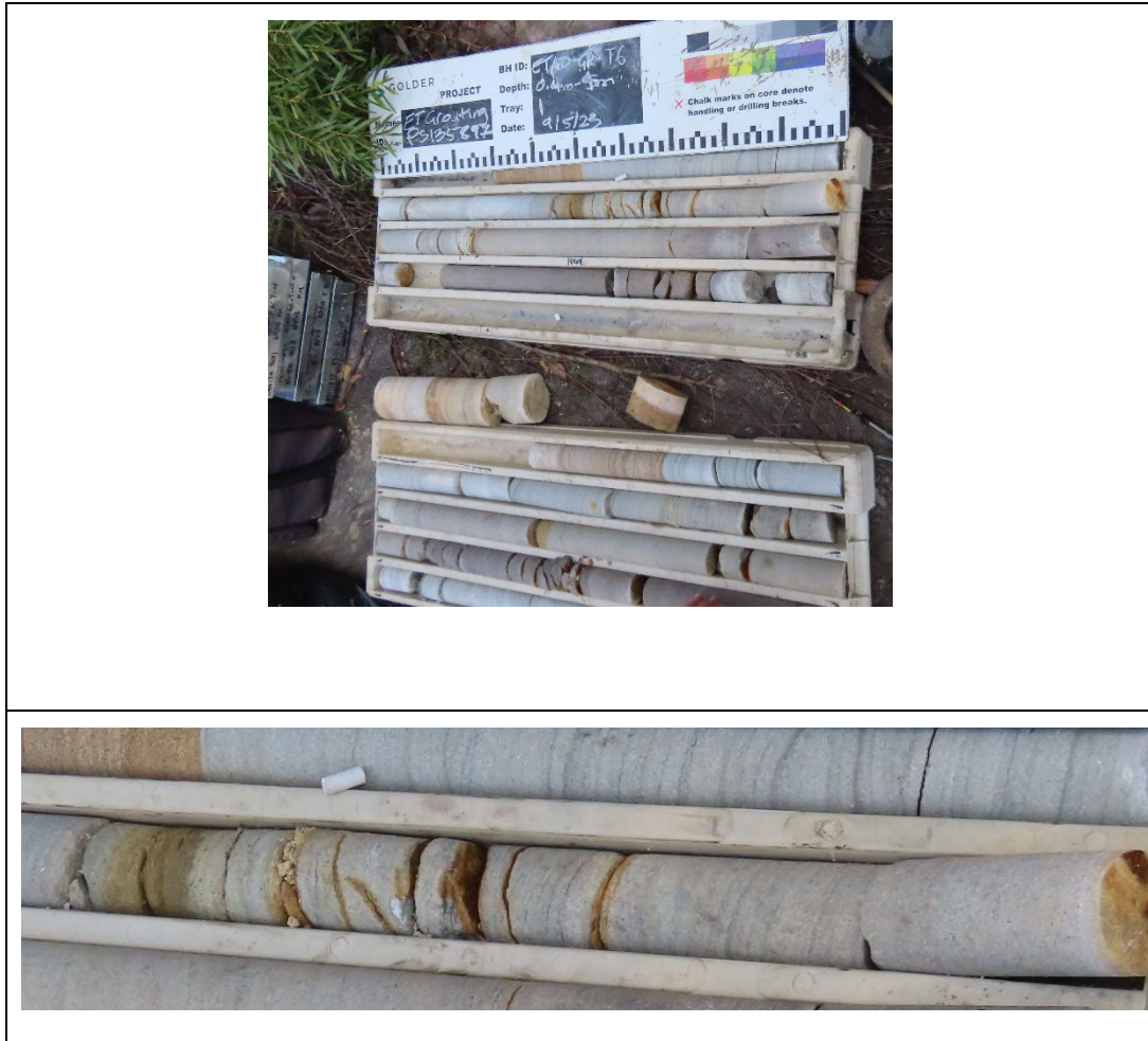
Figure 11: Core observed during the Panel's site visit on 10/5/23, the core having been recovered to a depth of 10 m from one side of Rockbar ETAO on the Eastern Tributary and showing a series of iron-stained partings indicative of subsurface flowpaths.
