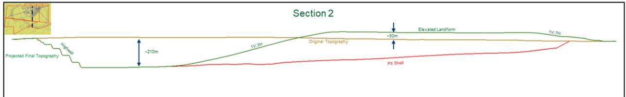
Figure 5: Section 2 – Partially backfilled pit and elevated waste dump to the south of the final pit
