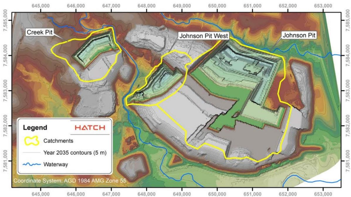
Figure 9: 2016 Study Final Landform and catchments considered for Void Water Balance Model
