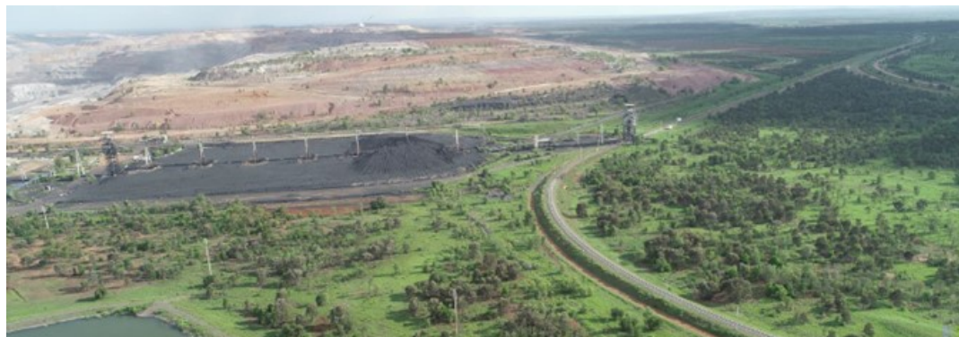
Figure 15-4. Product Stockpile and Loadout Facilities
